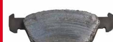
**Appearance.** The brake pad friction material is glazed
