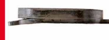
**Appearance.** A back plate that is damaged.
