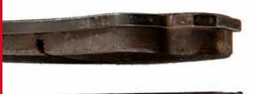
**Appearance.** One or more brake pads within an axle set is extremely worn.
