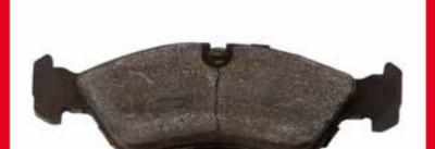
**Appearance.** Small cracks in the middle of the pad
