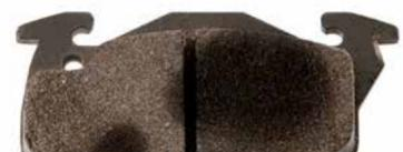
**Appearance.** Contamination of the Friction material with either oil, grease or brake fluid.
