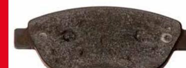
**Appearance.** The friction material is totally worn out.
