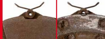
**Appearance.** Rust between the friction material and back plate.
