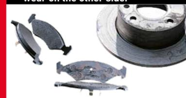
**What caused it?** One brake pad is in constant contact with disc. This causes the pad to wear down to the metal backplate.
