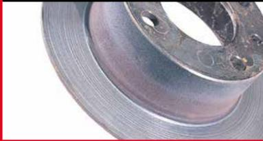
**What caused it?** Excessive or full brake pad wear results the brake pad backplate contacting the disc (metal to metal). This will make grooves in the disc surface.
