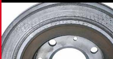
**What caused it?** Loose rough/sharp particles like dirt, road or water. Or badly mixed friction material between pads and disc.
