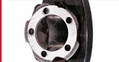
**What caused it?** Needless tightening and failure to observe recommended torque and sequence by the manufacturer during tightening.
