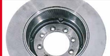
**What caused it?** Tightening sequence incorrect, not enough tightening torque used.
