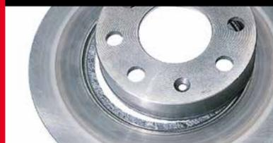
**What caused it?** Mechanical stress caused by misalignment and wrong assembly/positioning of the caliper and the disc. This causes asymmetrical wear of the braking surface.
