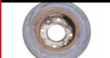
**What caused it?** Friction material deposits on disc surface. This usually appears where bad quality brake pads have been installed.
