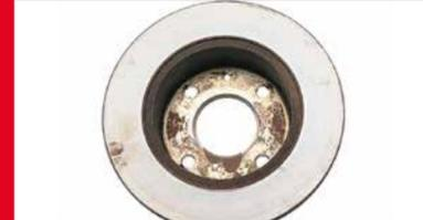
**What caused it?** Contamination on hub surface. This results in misalignment during mounting leading to irregular contact between pad and disc surfaces and irregular wear of the disc.
