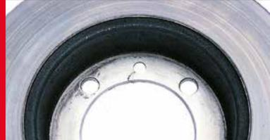
**What caused it?** Too much severe tightening torque used on positioning screw.
