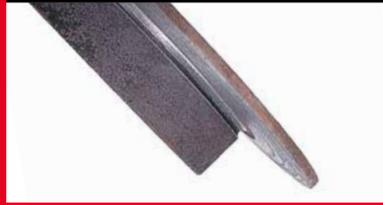
**What caused it?** Extreme pad and disc wear may result in movement of the backplate within caliper. In this case, the backplate of the worn pad has separated from its seat within caliper causing grooving between hat and disc surface.
