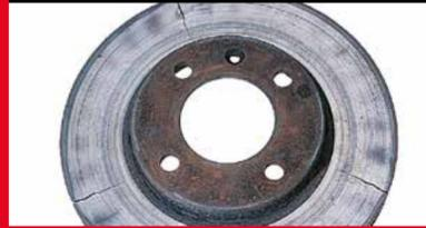
**What caused it?** Blue spots are a result of rising cracks caused by metallurgical change in the surface material making it hard and brittle. This is common in cases of overloading the brakes beyond normal design limits. This could result from aggressive driving, excessive payload or intensive/unusual brake use.
