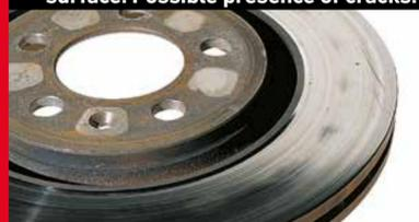
**What caused it?** Incorrect assembly of the caliper and/or pads can cause the pads being at a different angle to the disc, each side wearing at changed rates. Blue spots are generated by severe localized overheating.
