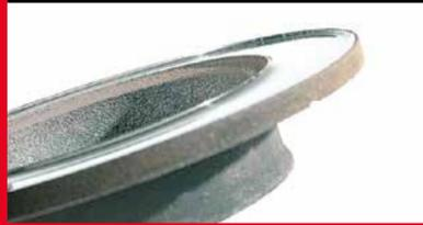
**What caused it?** Discs were not inspected regularly or replaced at the correct moment.
